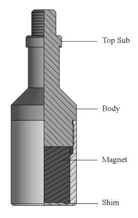
WARNING: Very powerful magnets are enclosed within the tool, and care should be taken to prevent damage to electronic equipment, and any materials in your shop.
